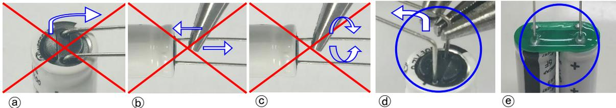
14. **(Radial type only)** NESSCAP recommends utilizing PCB when connecting Pseudocap to the circuit or electric devices. For best practice, avoid connecting wires directly to the Pseudocap devices and avoid locations near heat generating components.
