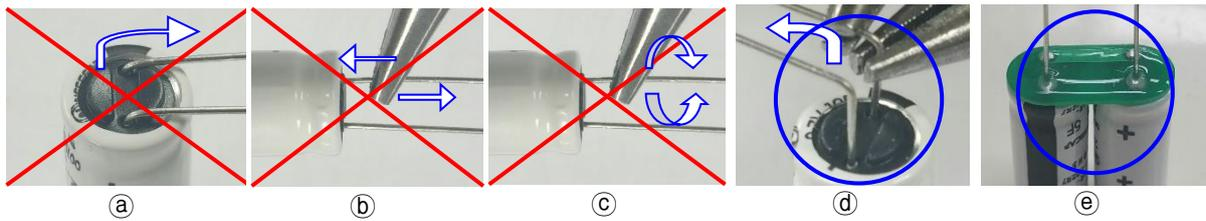
6. **(Radial type only)** NESSCAP recommends utilizing PCB when connecting EDLC to the circuit or electric devices. For best practice, avoid connecting wires directly to the EDLC devices and avoid locations near heat generating components.
